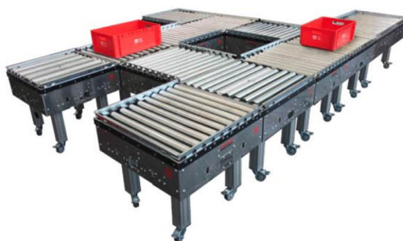
FIGURE 5.7 – Convoyeur modulaire [Soh et al.14]
